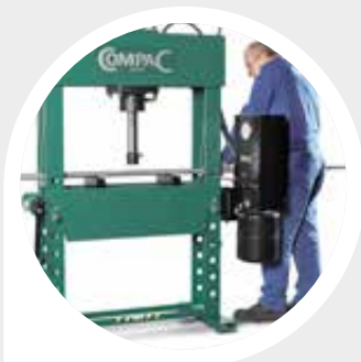
A 90° hinged pump unit enables easier insertion of longer work-pieces.
