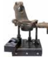
061248 Universal bearing removal support.
